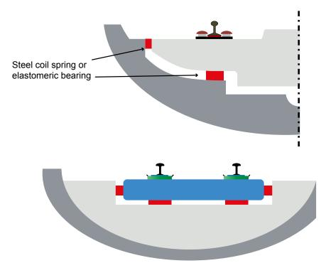
Graph 27. Floating slab in cylindrical tunnels. The mass of the slab including train and the spring rate of the bearing determine the resonance frequency of the single mass spring system.
