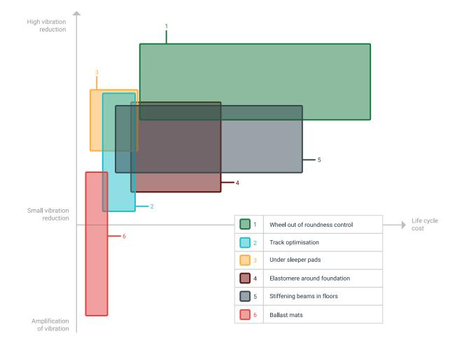
Graph 38. Comparison of mitigation measures suitable for application in existing tunnel situations. Annual simplified life-cycle cost for mitigation at a hot spot of 500 m length with 40 premises, and their effectiveness in terms of percentage reduced of the rms vibration velocity. A negative reduction means that there is a risk that the velocity will increase due to the measure being implemented.
