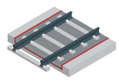
Graph 21. Under-ballast mat in a concrete trough or in a tunnel.
