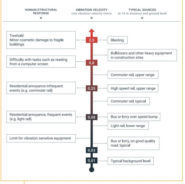
Graph 2. Typical sources of vibration with their typical strength. Adaptation from FTA-VA-90-1003-06, May 2006, transit noise and vibration impact assessment.
