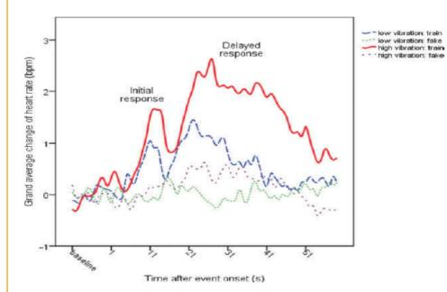
Graph 12. Heart rate change during sleep following freight train pass-bys with "low" (blue curve, 0.7 mm/s) and "high" (red curve, 1.4 mm/s) vibration strength. The levels applied here are hardly ever found in practice [3].
