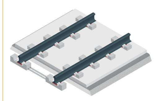
Graph 23. Non-ballasted track, with the rails being fixed in fixation blocks that are mounted on a concrete continuous slab (Rheda system).
