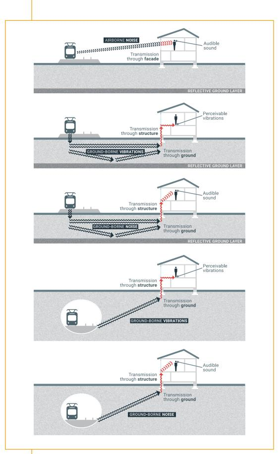
Graph 1. The different generating mechanisms and transmission paths of air-borne noise (not applicable for underground line), ground-borne vibration and ground-borne noise.
