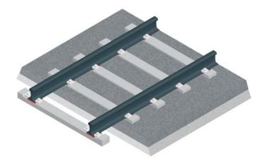
Graph 18. Schematic of regular ballasted track.
