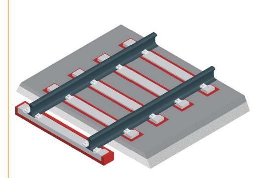
Graph 26. Slab track lost in the subsoil, with under-sleeper mat to make it into a floating slab.
