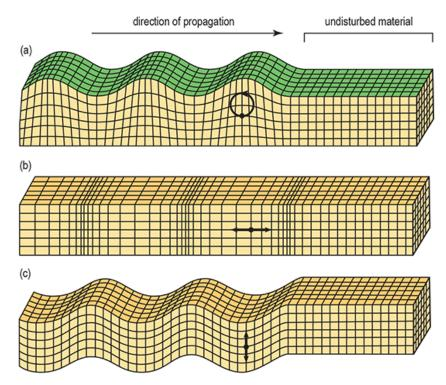
Graph 6. The three main wave forms in the ground association with the transmission of ground vibration [8].
