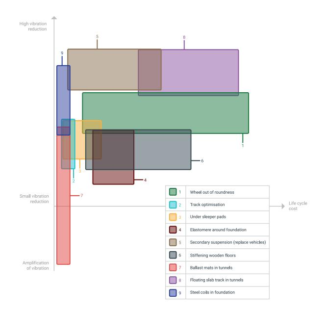
Graph 36. Comparison of mitigation measures suitable for application in new tunnel situations. Annual simplified life-cycle cost for mitigation at a hot spot of 500 m length with 40 premises, and their effectiveness in terms of percentage reduced of the rms vibration velocity.
