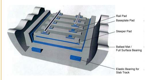
Graph 28. Slab track floating on elastomeric layers. © Getzner Werkstoffe GmbH.
