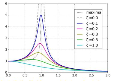
Graph 15. Simplified frequency behaviour of a single mass spring system with different damping factors  $\zeta$ . The main reduction is around the resonant frequency. The reduction is smaller, but at a wider range of frequencies, when the damping factor increases (source: Wikipedia).
