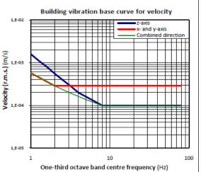
Graph 8. Building vibration base curves for just noticeable vibration expressed as acceleration (left-hand curve) or velocity (right-hand curve) for vertical and horizontal direction separately, as well as for the combined directions. After ISO 2631-2: 1989.
