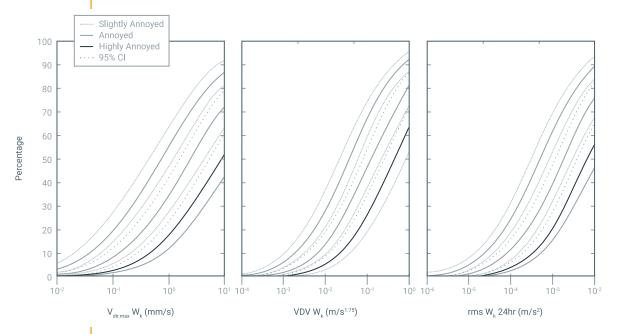
Graph 9. Exposure response curves following from a meta-analysis (total 4129 exposure and response data) carried out in Cargovibes [27]. The left-hand curve shows percentages of slightly annoyed, annoyed and highly annoyed residents as a function of the maximum weighted vibration velocity in mm/s.
