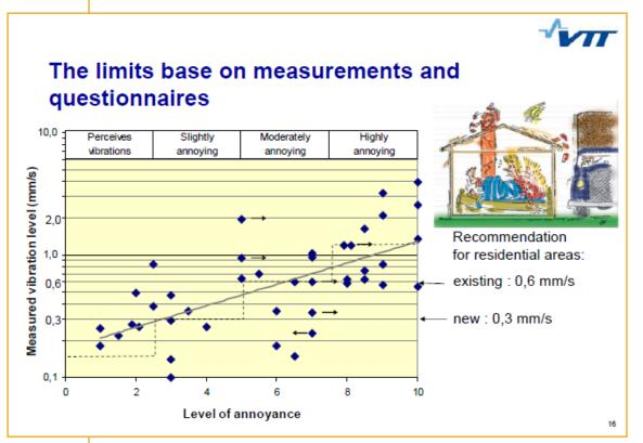
Graph 14. Illustration of recommended limit values derived from field survey and measurements (source: presentation by VTT).
