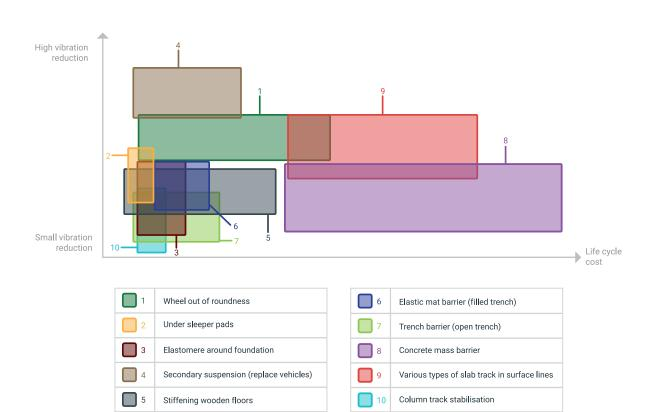
Graph 37. Comparison of mitigation measures suitable for application in new surface line situations. Annual simplified life-cycle cost for mitigation at a hot spot of 500 m length with 40 premises, and their effectiveness in terms of percentage reduced of the rms vibration velocity.
