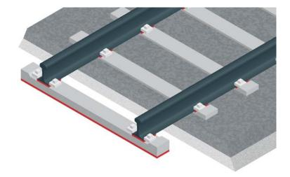
Graph 19. Under-sleeper pad for vibration reduction and ballast protection.
