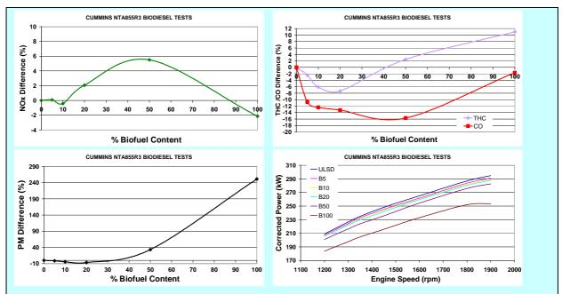
Figure 1: Initial results of UK bench trials of Biodiesel with the Cummins NTA855R3 engine, [Results are presented as % changes relative to ultra-low sulphur diesel fuel.]
