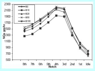
Figure 2: NOx emissions for Biodiesel blends
