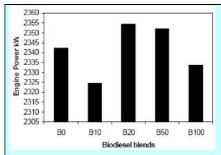
Figure 1: Maximum engine power for different Biodiesel blends
