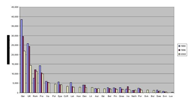
Figure 5: Liquid fuel consumption by EU 27 railways (1990, 1996, 2002)
