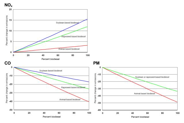
The US EPA study does also highlight that there can be important differences in the relative emissions performances of Biodiesel produced from different source oils, as illustrated in Figure 18. It could be expected that such variation will be somewhat reduced as a result of the definition of Biodiesel standards, such as the European Standard EN 14214 for Biodiesel produced from vegetable oils.
