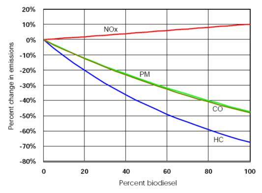
Figure 17: Average emission impacts of Biodiesel for heavy-duty highway engines (Source: US EPA<sup>53</sup>)
