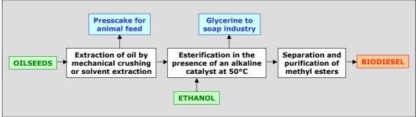
Figure 1: Production of Biodiesel by esterification of vegetable oil
