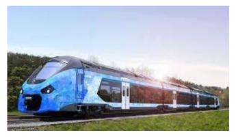
Train propelled by Hydrogen cells. Source: Alstom
